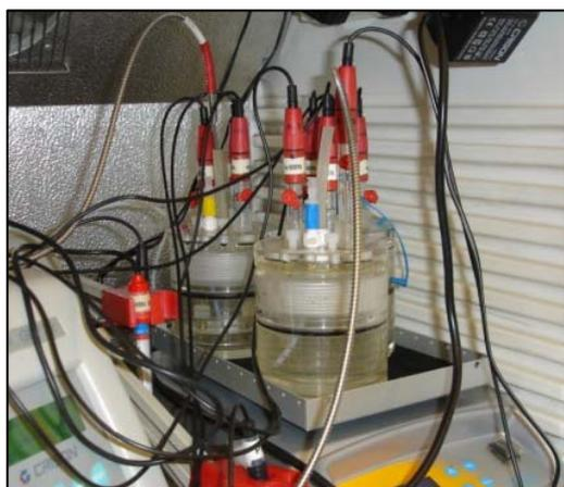
*Experiments of consumption of dissolved oxygen by mineral as a function of time (Domènech et al., 2011, 3<sup>rd</sup> ReCoty Annual Workshop)*
