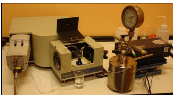
Autoclave used as a batch reactor to perform the solubility experiments and connected to TRLFS.
