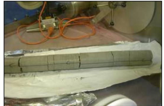
Core material of the Callovo-Oxfordian (EST30471) observed in anoxic glove box prior conditioning
