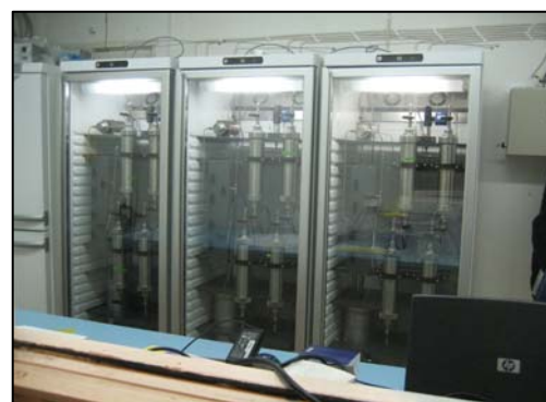
In situ circulations with flow cells for biofilm formation on crushed rock, with groundwater from -450 m (Photography from MICANS)
