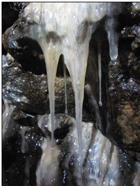
In the nuclear waste repository research tunnel ONKALO (Finland) massive biofilms are growing in a fracture zone. (Krawczyk-Bärsch et al. 2011, 3 rd ReCosy Annual Workshop)
